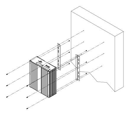
Using attached mounting rail, you can install AMI300 on wood, drywall surface over studs, or a solid concrete or metal plane. Ensure the installer uses at least four M4 length 8mm screws to secure the system on wall. Six M4 length 8mm screws are recommended to secure the system on wall.
